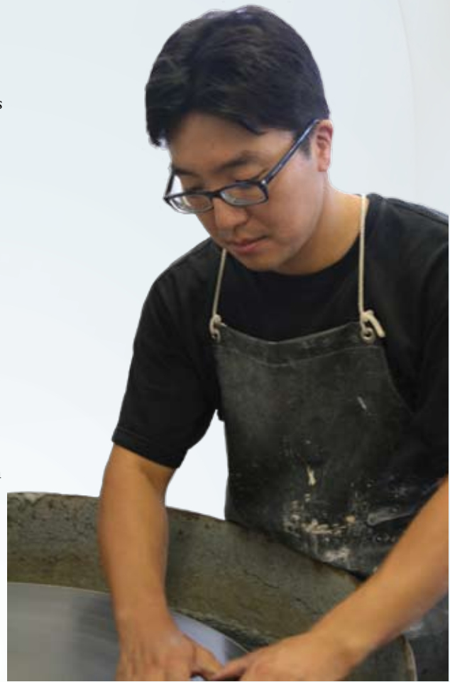
Jiyong Lee grinding glass parts on a flat silicon carbide grinder.
